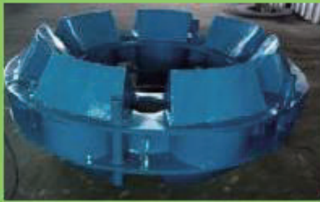
Load cell for bored pile
